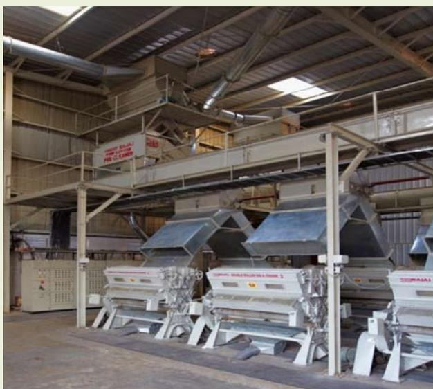
*Photograph of Central Screw Conveyor Distribution System
